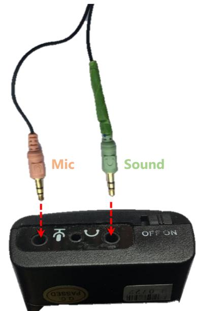
When turning on / off, if using the protective case it's advised that you remove the audio jack(s) from the device as pulling up the basal Velcro flap can bend and fatigue the wires (NB, the volume will also reset to minimum). UmpireTalk also recommends that you slide the on / off switch with the flat of your thumb instead of a fingernail.
